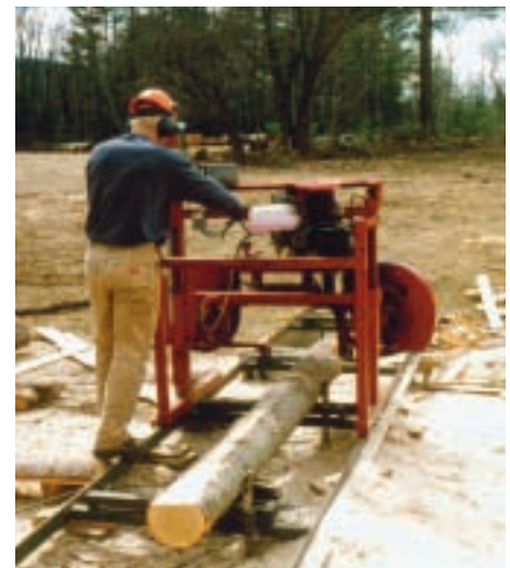
Gouge producing construction lumber from small logs cut on property.
